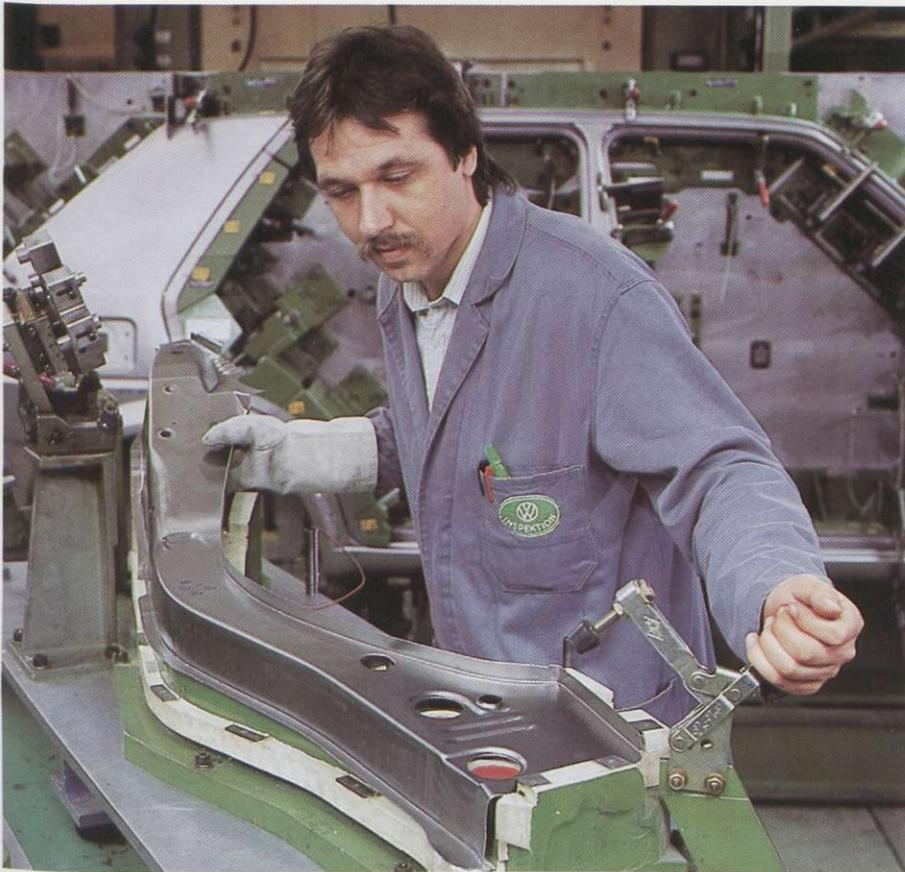
Parts being manually checked for dimensional accuracy
